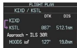
Figure 8-3 Active Flight Plan Window on the PFD
