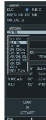
Figure 9-6 Selecting an Approach Procedure
