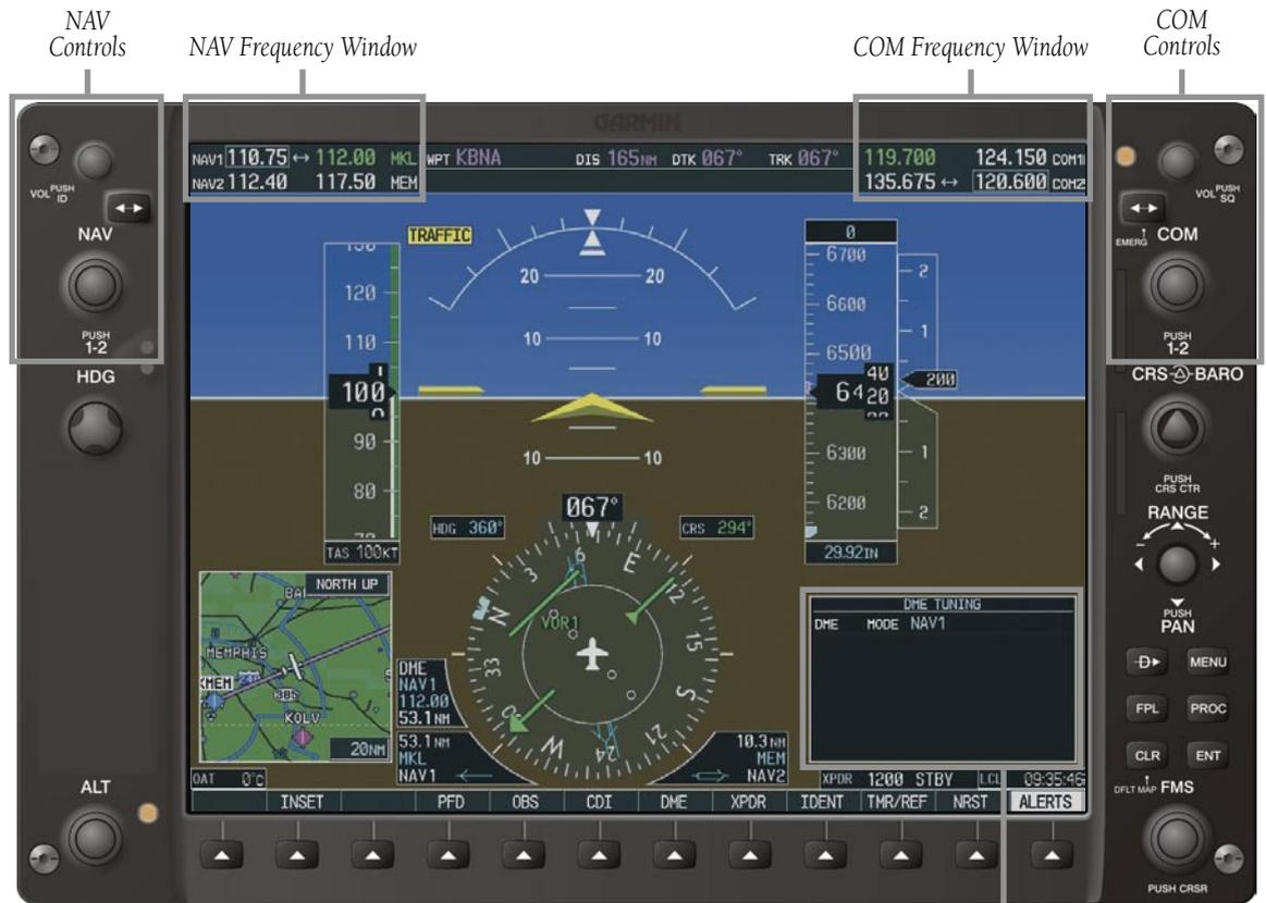
Figure 4-1 G1000 VHF NAV/COM Interface (PFD)
