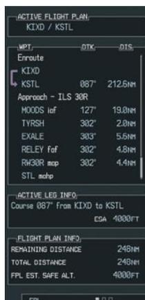
Figure 8-2 Active Flight Plan Page on the MFD
