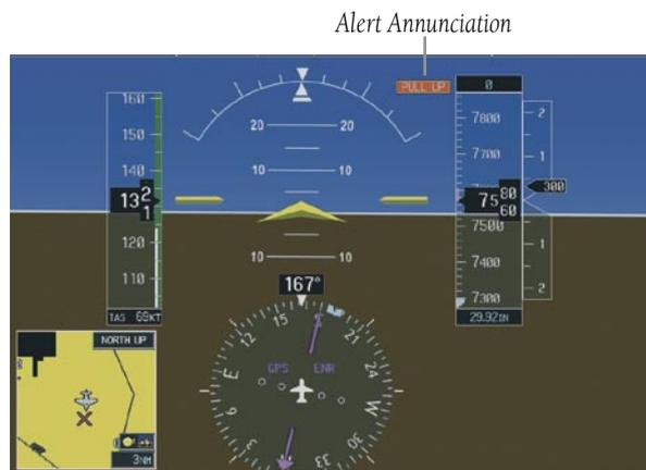
**Figure 10-28 Alert Annunciation on the PFD**
